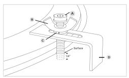
STEP 5 - ATTACH UNDERMOUNT CLIPS
